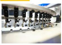
The functioning of the Computerized Jacquard Transfer Rib Knitting Machine combines Computerized Jacquard technology with Transfer Rib weaving. Various jacquard patterns can be easily produced and modified on this machine, allowing the users to keep up to speed with fashion trends. Sintelli's advanced computerized system ensures faster pattern color-changing.
