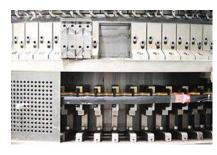
The double jersey electronic jacquard circular knitting machine features a computerized actuator to select needles on the cylinder. Any complicated structure/ design of fabric can be input into the special control system by computer, which can knit various designs of jacquard fabric. Professionally-designed high-speed CAM system
